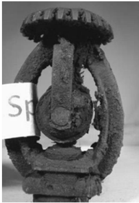
Sprinkler assembly has evidence of corrosion
